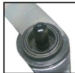
Detail of Internal sealed thrust bearing Quantum Crane "Z"
